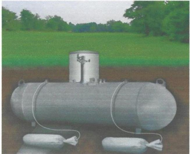
Although underground tanks are designed especially for this purpose, nature can corrode a steel tank that is not properly protected. It is important that you maintain and protect your tank against corrosion. The propane industry utilizes special underground tanks that are manufactured with a preventive coating. In addition underground tanks are protected by a process called “Cathodic Protection.”
